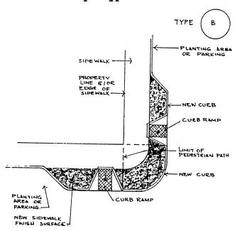
(1) This curb ramp type can be used with the existing planting area or with the sidewalk extension into the parking area.
